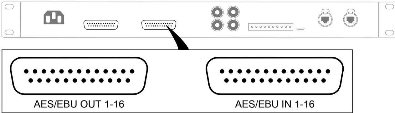
The connectors are wired according to the AES59 8-way pinout annex C standard.
