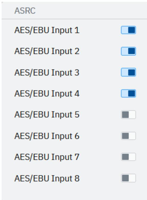
Turning off the ASRC can be used to propagate a particular clock domain from an AES/EBU input, or if all AES/EBU inputs are on the same clock.
