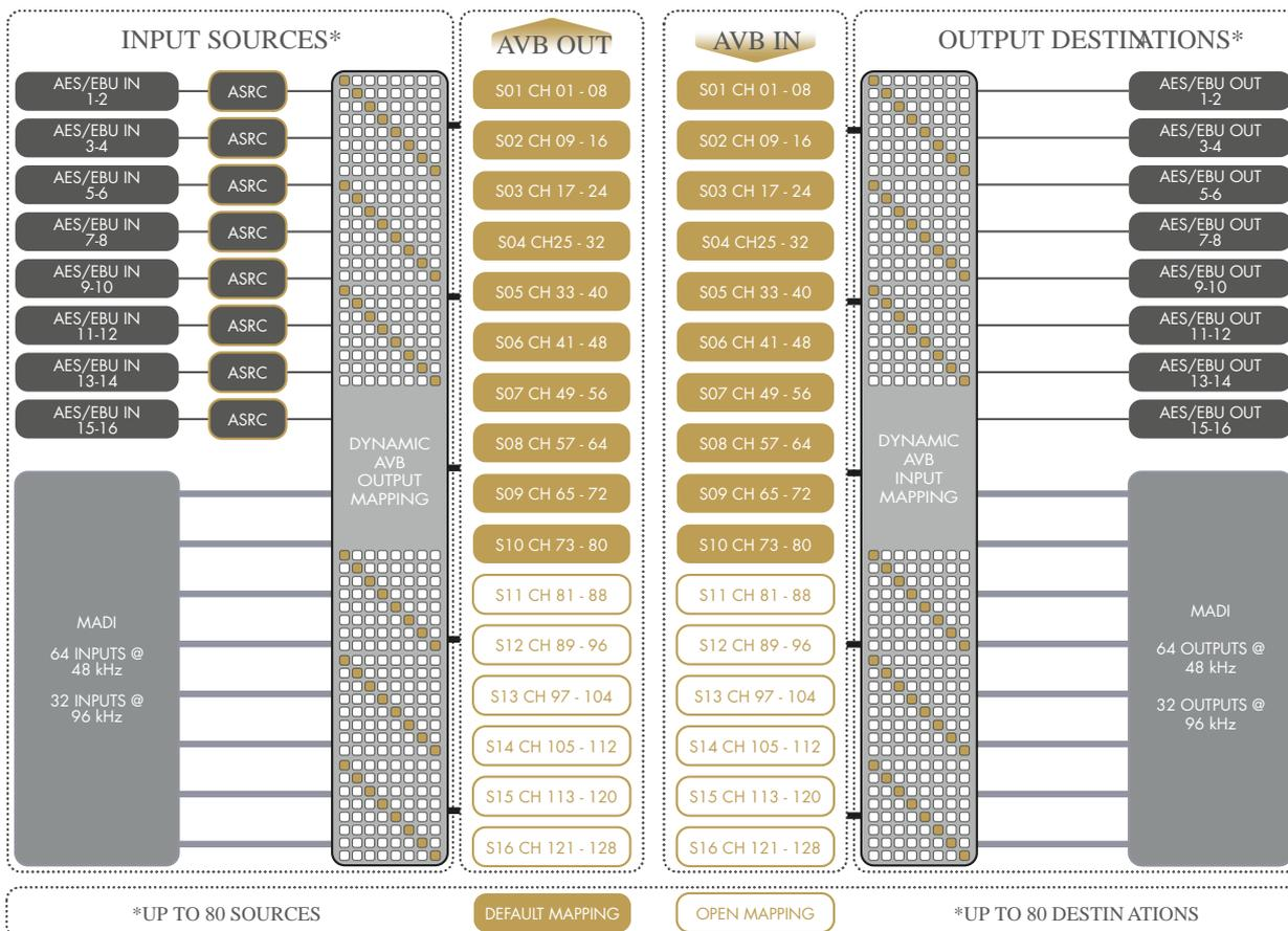
Mapping is possible from the Milan-AVB inputs to the AES/EBU and MADI outputs, and from the AES/EBU and MADI inputs to the Milan-AVB outputs. Direct mapping between Milan-AVB inputs and outputs is not possible, neither is it possible to map between AES/EBU and MADI.
