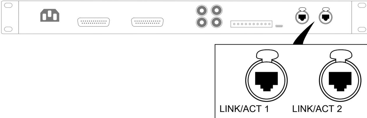
In normal network mode, the two etherCON connectors are part of an internal Milan-AVB switch.
