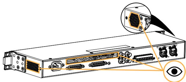
rear and side grills and clean are not damaged
