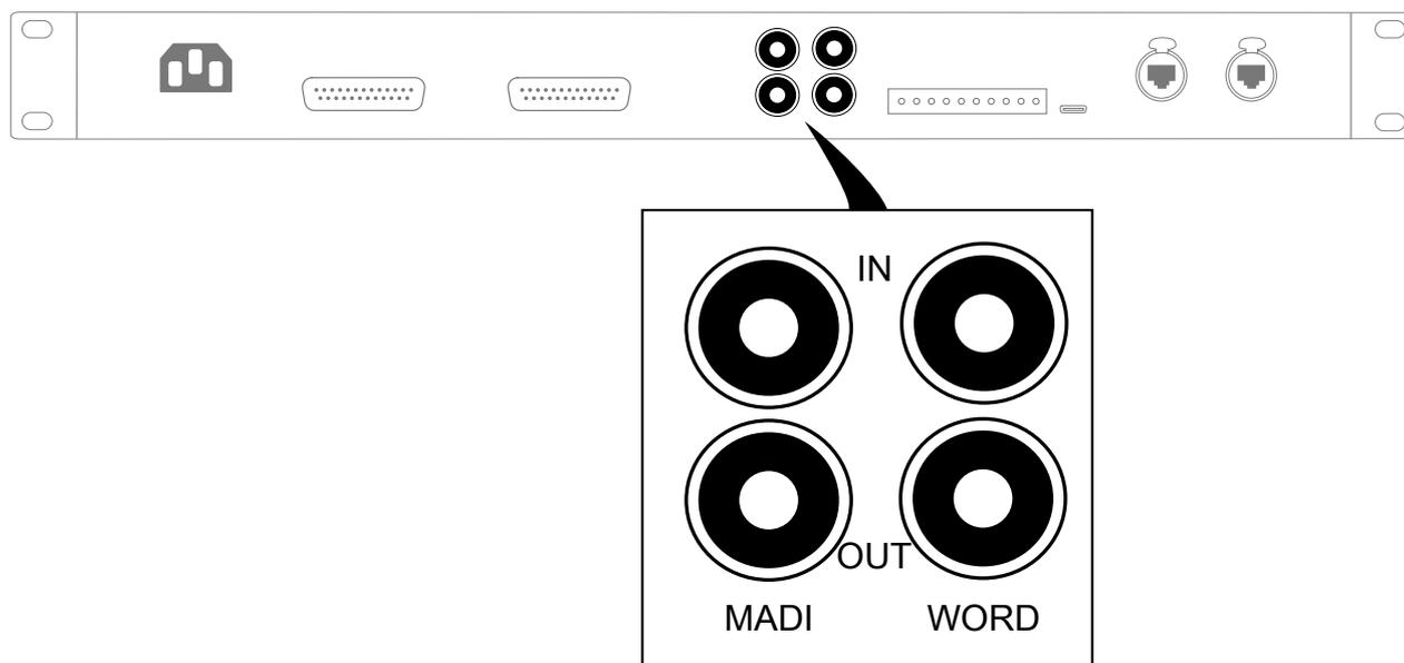
**MADI IN** can receive up to 64 AES10 digital audio signals at 48 kHz or 32 AES10 digital audio signals at 96 kHz. There is no sample rate conversion. The default mapping is to output streams 3 to 10 (at 48 kHz) or to output streams 3 to 6 (at 96 kHz).
