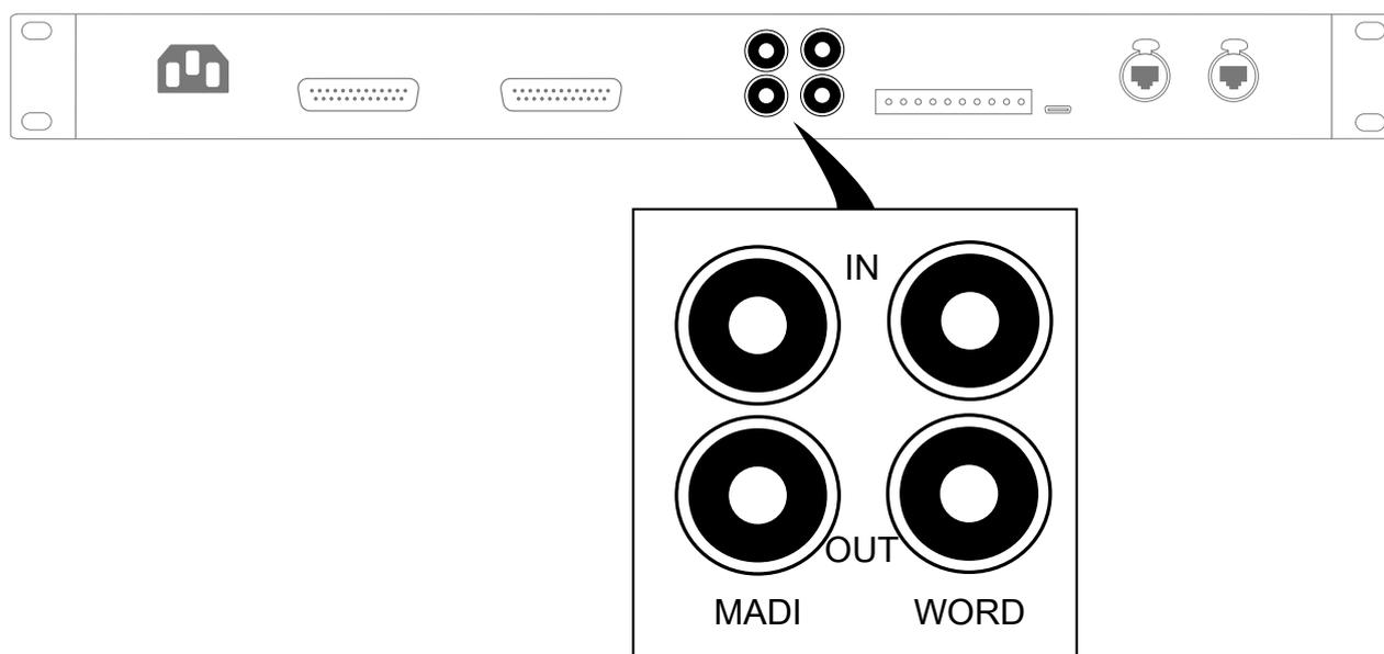
The supported input frequency is 48 kHz or 96 kHz. **WORD IN** accepts input levels from 1 V<sub>pp</sub> to 5 V<sub>pp</sub>, and is protected from overvoltage. **WORD OUT** output level is 5 V<sub>pp</sub> into open load.
