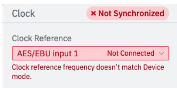
If the selected clock reference is lost, a warning is displayed and LC16D operates in "freewheel" mode. Audio at the same sampling frequency is transmitted but there can be small glitches in the audio as the phase drifts between the clocks. A valid clock reference that matches the audio signals should be selected.
