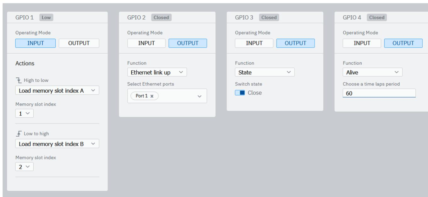
LC16D GPIO connector has four pins available either as input or output.
