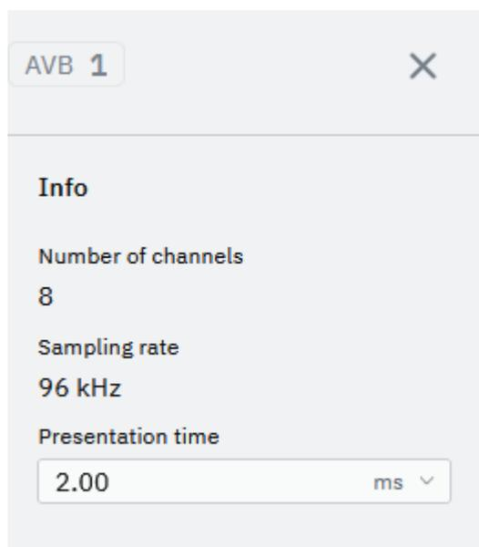
The selection of the presentation time can be unavailable if the stream is already connected or if LC16D is locked by an AVB controller (such as **Hive**).
